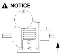
• Lubricating oil should be filled to the center of oil gauge while the unit is not running.
