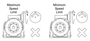
◆ Do not turn hand wheel when the unit is not running.
