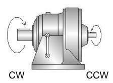
Double Reduction, 102:1 ~ 7569:1 Output Direction = Input Direction
