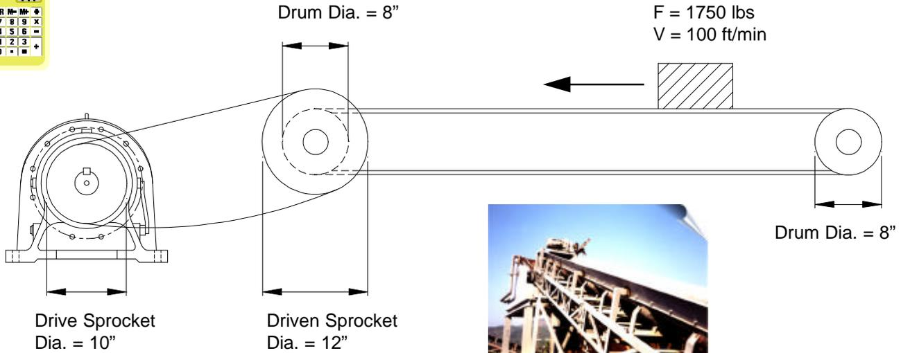
You are designing a conveyor driven by a gearmotor. The conveyor has a 1750 lbs force acting on it, and moves at the speed of 100 feet per minute. This conveyor will operate at 10 hours per day with moderate shock load. Please select the appropriate DARALI®DRIVES frame size and reduction ratio.
